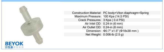
The ozone check valves are an important component in preventing damage to the ozone generator. BEYOKozone valve assemblies are designed to be used in conjunction with the ozone generators to avoid back flow.
