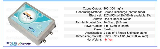
The BEYOKozone FM- series ozone generators are highly integrated corona discharge three in one units with ozone tube, ozone power and air pump in one plastic case (FM-300SNP without air pump). They have been used as a functional unit for residential air sterilizers and for water treatment, including applying to spas, baths, small pools and anywhere small volume of water sterilizing.
