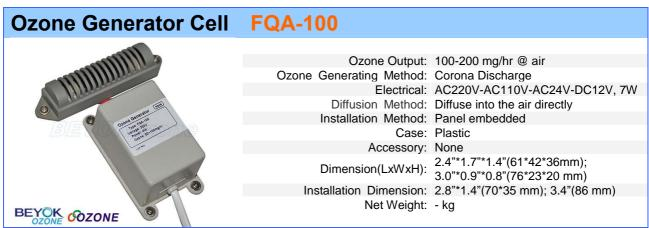
The FQA- series of BEYOK ozone generator cells are mainly used for air disinfections and sterilizations with panel embedded way, they can provide stable and efficient ozone output, easy to install, operate and maintain.
