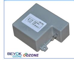
Ozone Output:100-200 mg/hr @ airExternal gas source:1-5L/min@air; 0.5-2L/min@oxygenOzone Generating Method<br/>Electrical:Corona Discharge<br/>AC220V-AC110V-AC24V-DC12V, 5WOzone Outlet Connection:Φ 6mm pagoda joint<br/>PlasticCase:PlasticDimension(LxWxH):3.1"\*2.6"\*1.3" (80\*67\*33 mm)Installation Dimension(LxW):2.8"\*1.6"(70\*40 mm)<br/>Net Weight:
