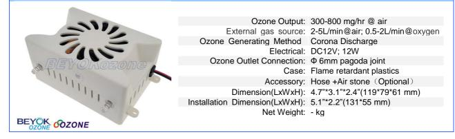
The FQT-series of BEYOK ozone generator cells use ozone core discharge of invention patent, including the integration design of ozone generator tube and ozone driving circuit (without air pump), they can provide stable and efficient ozone output, easy to install and maintain.
