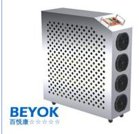
Ozone Output:120 g/hrOzone Generating Method:Surface Corona DischargeElectrical:220V/50Hz-120V/60Hz, 1520WOzone concentration:Max.10-20 mg/LControl:Electronic loop controllerAccessory:N/AApplication Range:600-1000 m2Case:Stainless steelDimension(LxWxH):33.5"\*11.8" \*23.6" (850\*300\*600mm)Net Weight:42 kg
