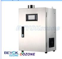
Ozone Output:20 g/hr; 40ppmOzone Generating Method:Sheet Multi-Group Air Gap DischargeElectrical:220V/50Hz, 200WAir volume:300m3/hControl:Programmable controllerInstall method:Floor or back hangingApplication Range:400-600 m3Case:Stainless steelDimension(LxWxH):15.7"\*10.8"\*25.6" (400\*300\*650 mm)Net Weight:17 kg
