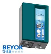
Ozone Output:20 g/hr@5Lpm O2 externalOzone Generating Method:Corona DischargeElectrical:220V/50Hz-120V/60Hz, 180WGas Source Input:Connect to external gas sourceControl:Outside connect to system control boardCooling Method:Air cooledInlet & Outlet Connection:0.3"\*0.2"(8\*6mm)Stainless steelCase:MetalDimension(LxWxH):11.8" \*6.7" \*18.9" (300\*170\*480 mm)Net Weight:-lbs (- kg)Adapted swimming pool:300m3
