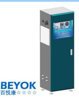
Ozone Output:200g/hr@40Lpm O2 externalOzone Generating Method:Corona DischargeElectrical:220V/50Hz-120V/60Hz, 1600WGas Source Input:Connect to external gas sourceControl:Programmable electronic loop controllerInlet & Outlet Connection:0.3"\*0.2"(8\*6mm) Stainless steel& HoseCooling Method:Water cooledCase:Stainless steelDimension(LxWxH):15.7" \*13.8" \*39.4" (400\*350\*1000 mm)Net Weight:-lbs (- kg)Adapted swimming pool:2500m3
