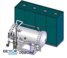
Ozone Output:10kg/h@ dry oxygen enriched air<br/>Electrical:Block380V/50Hz, 75KWInput air source:External oxygen enriched system, 80Nm3/h<br/>Cooling Water:Cooling Water:External Cooling Water, 20 T/h<br/>Ozone can be adjusted (PLC controller)Air Inlet& Outlet:DN40 Stainless Steel FlangeWater Inlet & Outlet:DN50 PVC Pipe Flange<br/>Main Materials:Dimension(LxWxH):110" \*91" \*79" (2800\*2300\*2000 mm)<br/>Net Weight:
