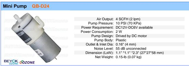
BEYOKozone Mini Pump MPD-24A use a DC power motor design that has the capability of over 18,000 hours of continuous maintenance-free operation. It is compact, very quiet, highly reliable and inexpensive.
